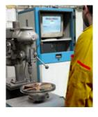
Pulleys balanced on electronic balance machinery, cooling fins designed to operate with optimum efficiency.
